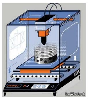
then lowered fractionally and the next layer added. Another way is fused deposition modelling, a system used by Stratasys, a company based in Minneapolis. This involves melting plastic in an extrusion head to deposit a thin filament of material to build the layers.
